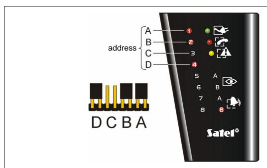
Fig. 3. Setting of the jumpers and corresponding LEDs during programming procedure in the CA-6 KLED keypad
